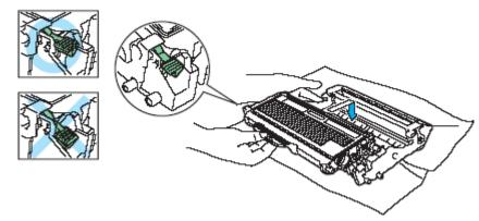
6. Put the drum unit and toner cartridge assembly back in the printer.
