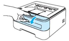
2. Slowly but firmly pull the drum unit and toner cartridge assembly out of the machine.
