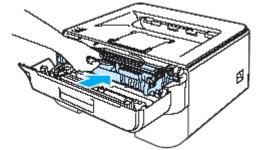
7. Reset the drum counter. Press and hold down the white button (shown as blue in the image below) for about 4 seconds until all the LEDs light up. Once all 4 LEDs are lit, release the button.
